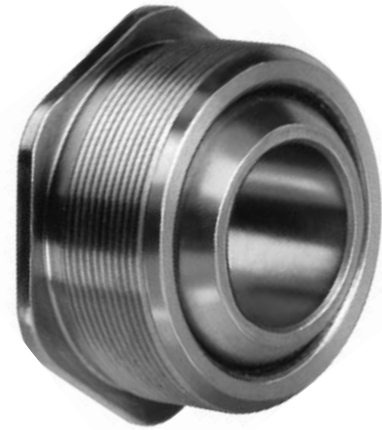
This aircraft flanged spherical bearing uses a threaded O.D. to provide a retention feature. The threaded O.D. also allows for ease of replacement in the application.
