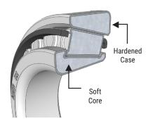
NTN also offers TRBs with through-hardened steel, including many of our ISO TRBs, for applications requiring less shock load capabilities as a cost-competitive alternative.
