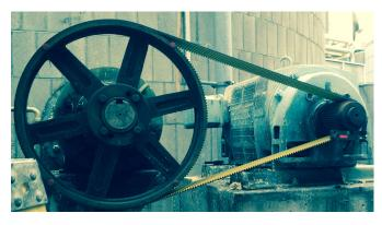
Narrowing the belt drive width will move the hub load closer to the bearing. Moving the pulley as close to the bearing as possible will reduce hub loads on both bearings. Hub load reduction will improve bearing life and is significant in saving downtime and replacement costs.
