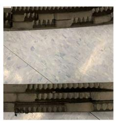
5VX is EPDM which can withstand heat up to +230degF (most resistant Continental belt to heat). The "X" clarifies that the belt is cogged and more flexible around smaller pulleys compared to 5V wrapped belts. Pending a MaximizerPro drive analysis, below are common system application issues to look for with noticeable fatigue cracking:
